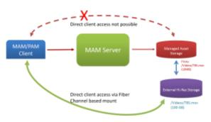
One strategy for coping with bandwidth limitations of Ethernet-based LAN is to use Fiber channel connectivity or a hybrid scheme. Fiber channel-based connection will avoid packet loss & transmission issues that can plague shared Ethernet connections, thus lowering latency and guaranteeing sustained throughputs to the storage directly.
